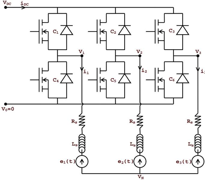
Fig. 6. Three phase inverter topology and starter-generator model
