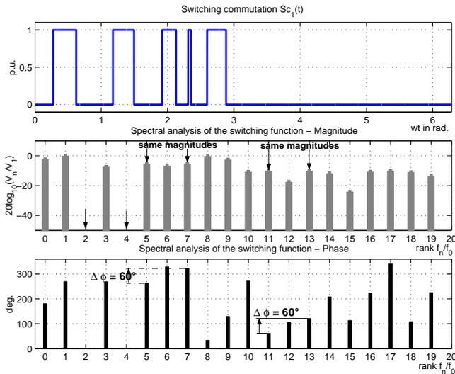
Fig. 8. Solution of the example with a general wave - switching function
