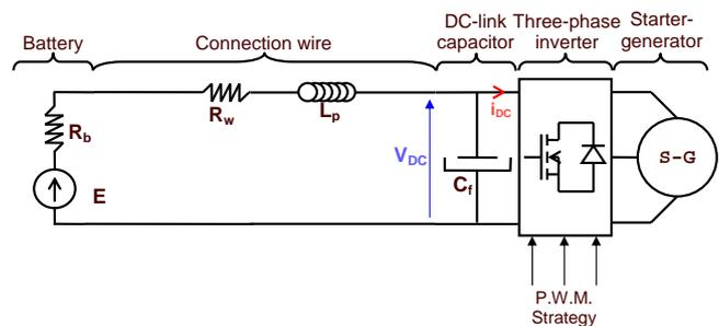
Fig. 1. Simplified electrical architecture
