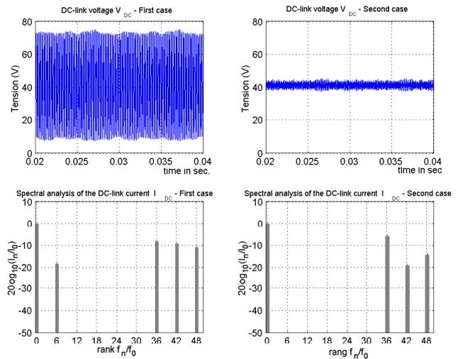
Fig. 10. Control of the DC-link voltage ripple
