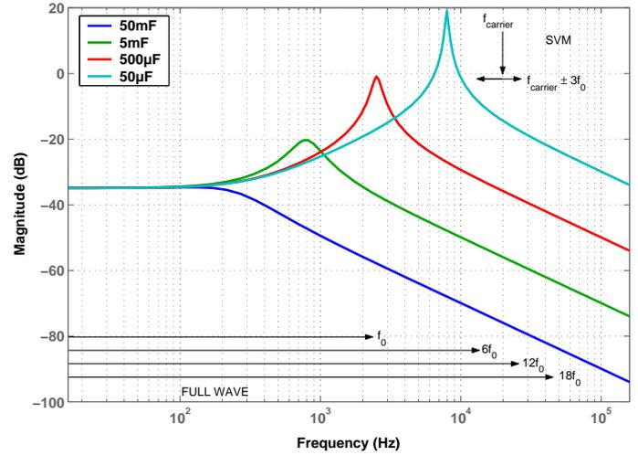
Fig. 5.  $i_{DC}$  harmonics range for full-wave modulation and SVM
