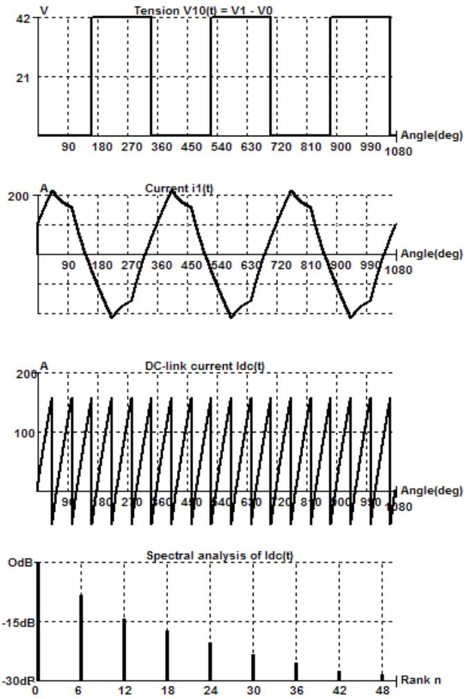
Fig. 3. Full-wave typical waveforms
