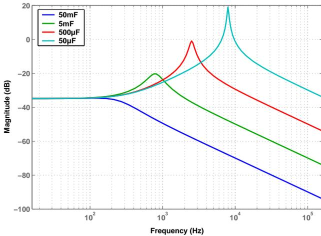
Fig. 2. Bode diagram of the transfer function for different capacitances  $C_f$
