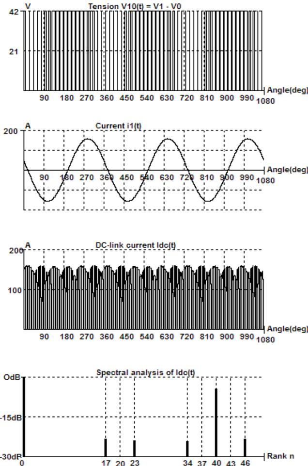
Fig. 4. SVM typical waveforms (frequency ratio  $R = 20$ )
