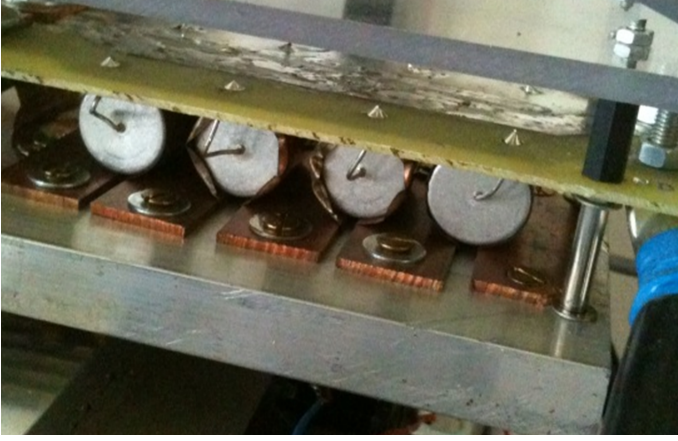
Figure 8. Electrolytic capacitors mounted on the thermal dissipator
