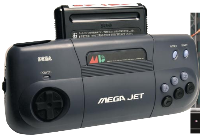
Avoiding any additional cables the Mega Jet was a combination of pad and console, designed for in-flight use.
