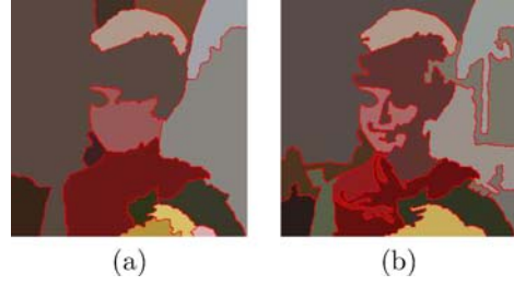
Figure 10. The same image segmented into 15 regions with a) a boundary length-based regularizer (Mumford-Shah), and b) a number-of-regions-based regularizer.
