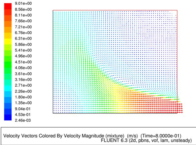
Figure 7: Velocity Vectors Colored By Velocity Magnitude after 80 Time Steps
