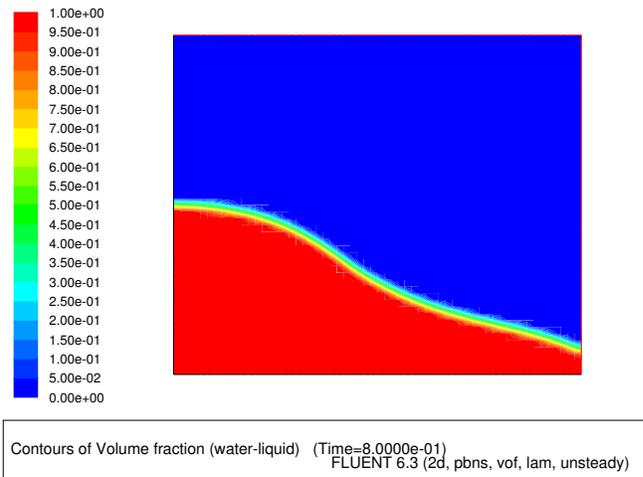
Figure 8: Contours of Water Volume Fraction after 80 Time Steps
