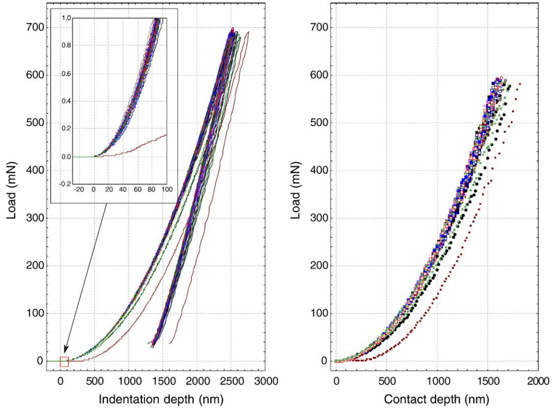
Fig. 1. 98 initial load–displacement curves on fused silica (left) and load–displacement curves after statistical pre-treatments using Oliver and Pharr method (right).
