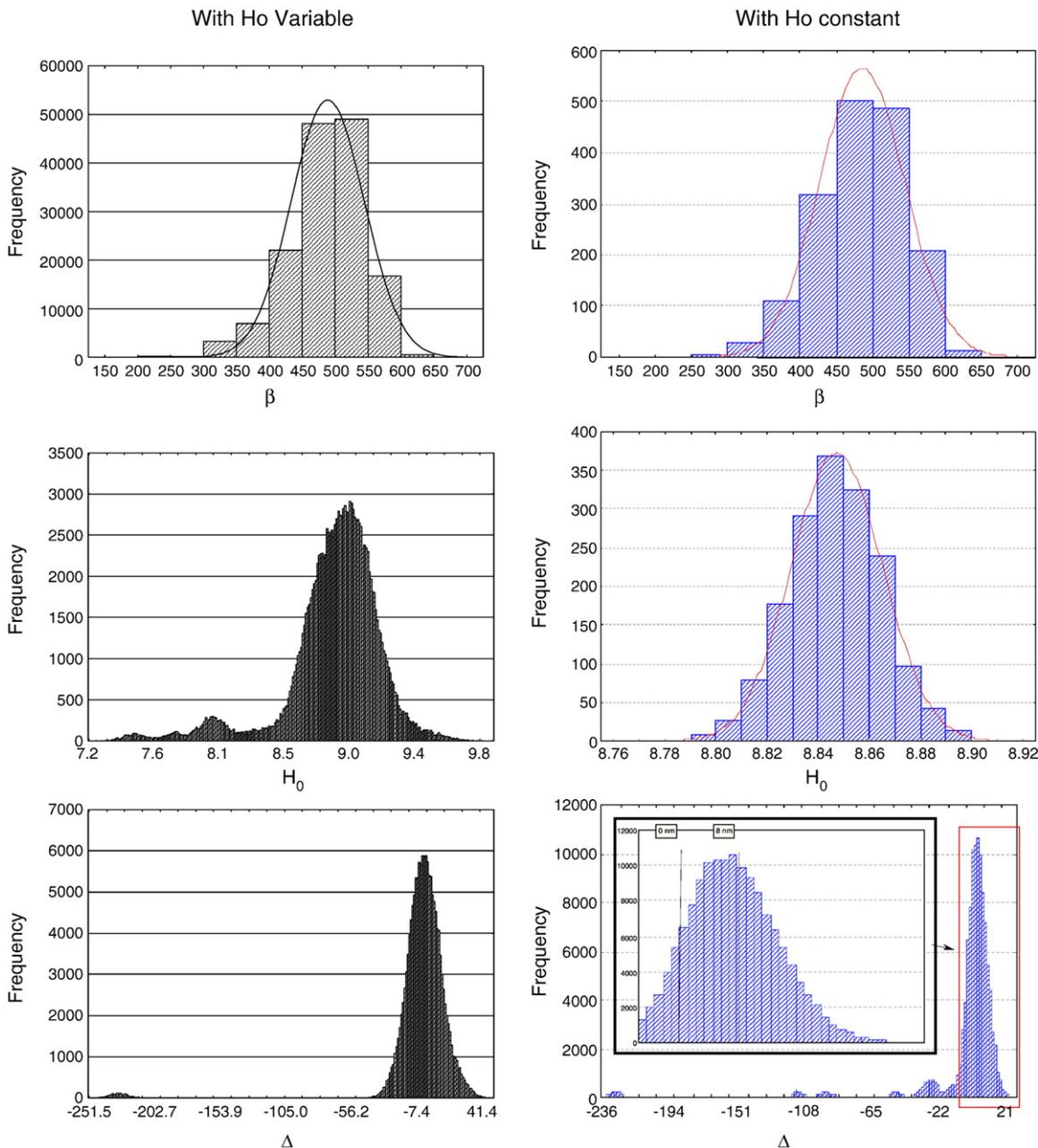
Fig. 2. Histograms of ( $H_0$ ,  $\Delta$ ,  $\beta$ ) when they are estimated from models given by Eq. (10) (left) and Eq. (11) (right).
