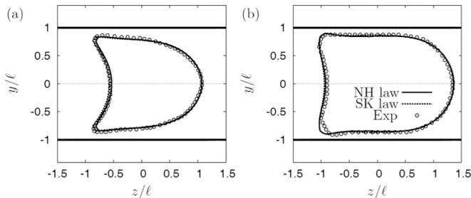
FIG. 9. Superposition of experimental and numerical capsule profiles in square-section microfluidic channel. The numerical profiles are obtained with the NH law or with the SK ( $C = 1.0$ ) law. (a) NH law ( $Ca = 0.08, a/\ell = 0.90$ ) and SK law ( $Ca = 0.17, a/\ell = 0.90$ ); (b) NH law ( $Ca = 0.03, a/\ell = 1.10$ ), and SK law ( $Ca = 0.05, a/\ell = 1.09$ ).
