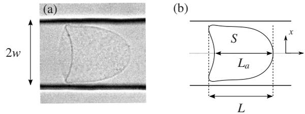
Fig. 3. (a) Experimental capsule profile in a specified  $50 \times 50 \mu\text{m}^2$  channel. (b) Numerical deformed profile in the plane  $y = 0$ ,  $L_p = L - L_a$ ,  $S$  is the contour surface area.
