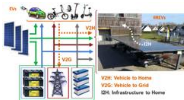
PV-powered electric vehicles charging station based on microgrid (30 Wp)
